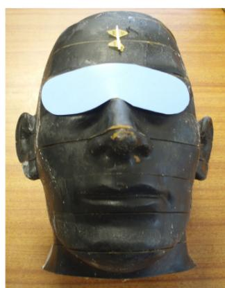
**Figure 3.** Rando head phantom with small shield in-situ
