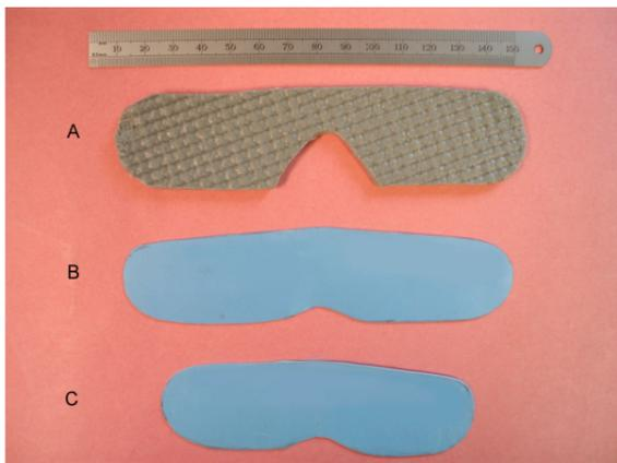
**Figure 1.** Foam "stand-off" (A) large barium vinyl shield (B) and small barium vinyl shield (C)
