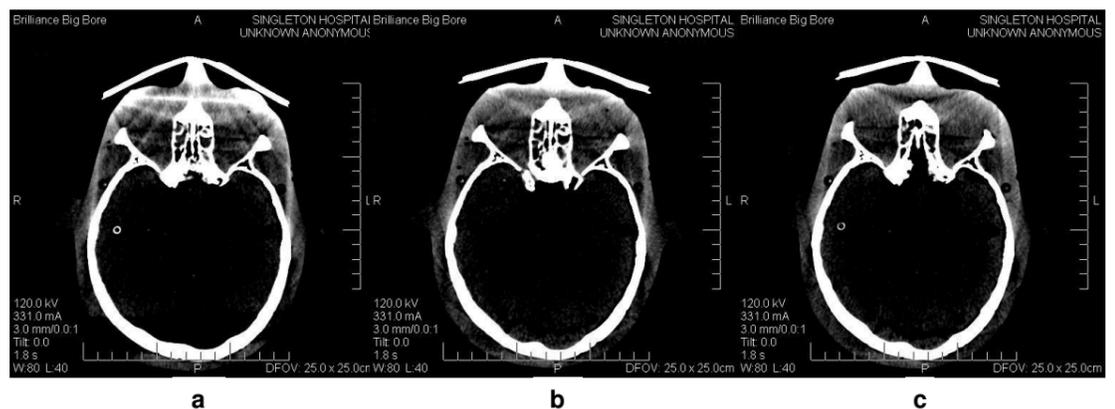
**Figure 4.** CT images showing image artefacts in the anterior region of the Rando head phantom with the use of large shield (a) large shield with foam "stand-off" (b) and small shield with foam "stand-off" (c).
